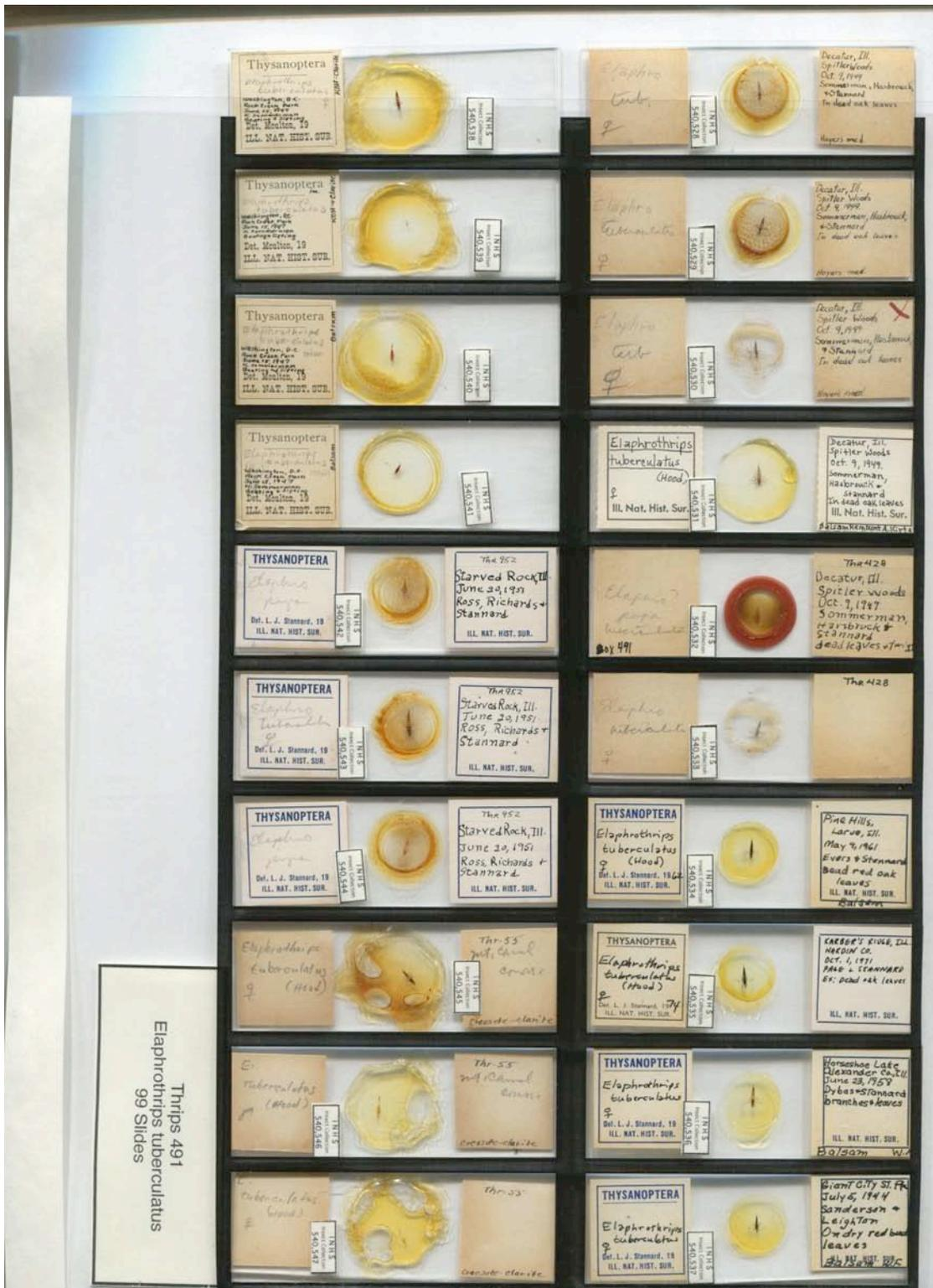
Set of 20 slides scanned using acetate film template (see next page). Spacing of slides is the same as for Plexiglas tray. Note that template is smaller than scanner bed and must be pushed to upper left corner of scanner bed (lower left in above image) to provide consistent results.
